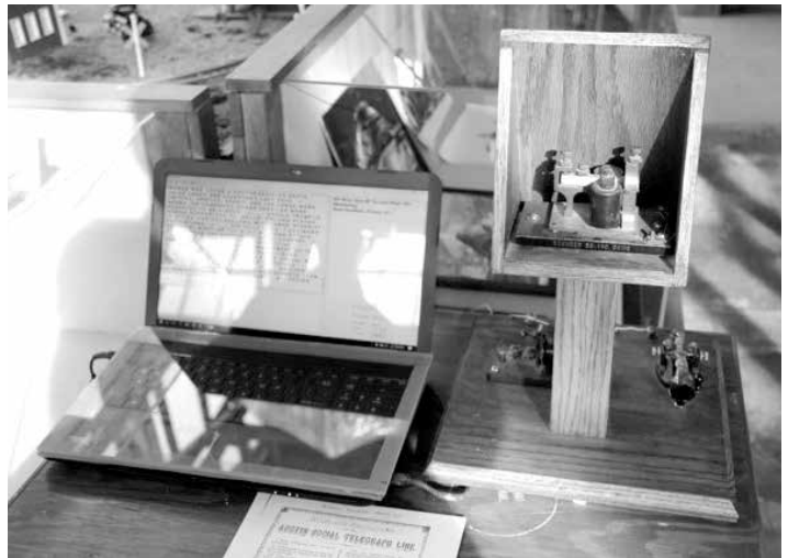
MorseKOB operating desk in the railroad heritage exhibit at the Foss Waterway Seaport museum. The MorseKOB news wire typically runs on the computer and sounder 24 hours a day, seven days a week ("Moon Yard, Tacoma"). A plexiglas cover discourages visitor hands on the keyboard of the notebook computer.
